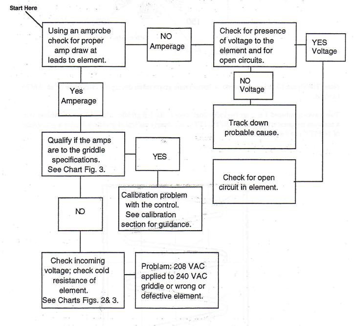
The most common problems with electric heating elements are open connections, bad connections, short circuits or ground faults. A grounded or shorted element will normally trip a breaker. In some circumstances, the grounded element can continue to heat without tripping a breaker.
